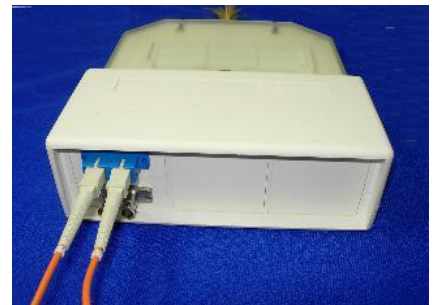
Step 6: Place back the cover and plug-in patch cords as needed.
