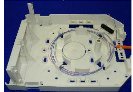
Step 3: Tie the cable to the box and wrap the fibers around the center 2~3 times as shown.
