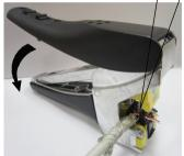
Insert the jack into the guide in either direction. Press tool to terminate the jack and cut off the excess wires.
