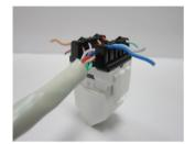
Press the wires through the slots.
