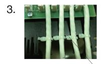
Step 3: Secure the cables to the cable bracket using the cable ties provided.
